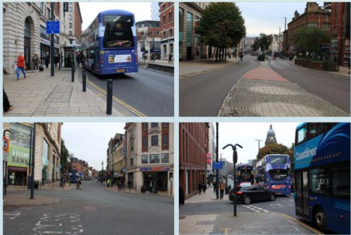
Figure 4: A selection of problems on the Headrow Gateway (clockwise from top-left: inadequate bus lay-bys; outdated landscaping and surfacing materials; buses delayed by general traffic; staggered pedestrian crossings and guard rails)
